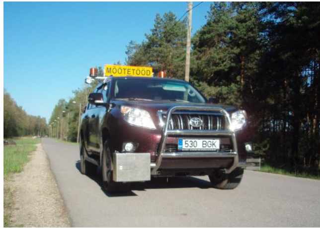
Fig. 1. Equipment for pavement texture and roughness measurement Laser Texture Meter LTM-1
