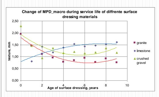
Pavements, surface dressed with granite and graded crushed gravel, are behaving similarly—texture values are decreasing during the service life.
