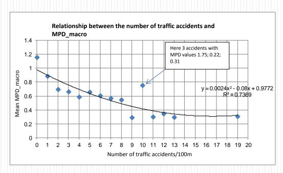
Traffic accident data form past 10 years was compared with pavement texture values. With the decrease of pavement macrotexture values the probability of traffic accident is clearly increasing.
