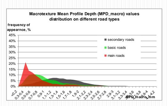
Lower macrotexture values were observed on main roads pavement, higher values were observed on secondary road pavement. Medium values are characteristic for basic roads. Similar distribution could be noted for megatexture values.
